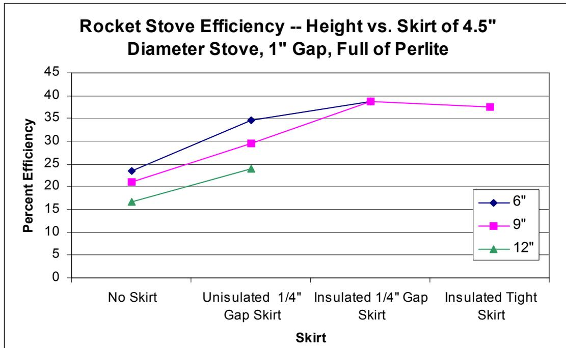
Use of the tight skirt, however, caused the efficiency to decrease by a few percent because of the problem of a lack of draft space for the exit air.
