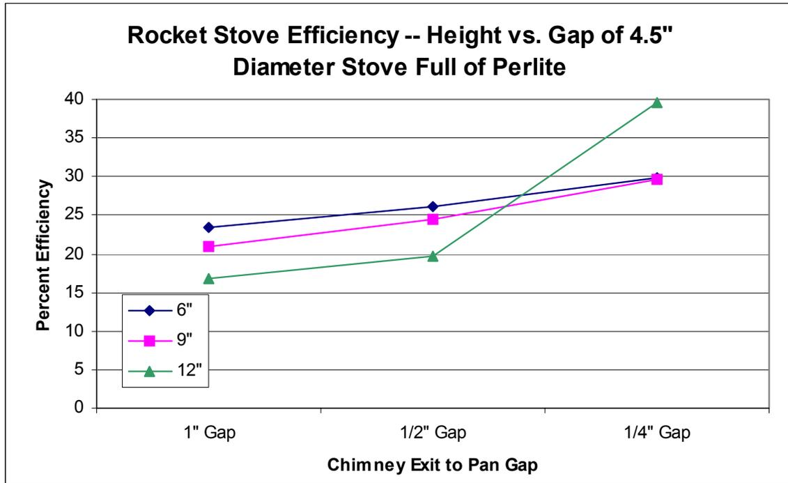
An important consideration, however, is that the 1/4" gap sometimes caused the fire to burn out the top front of the feed magazine because not enough air was able to be drawn through the decreased gap to create the proper draft.
